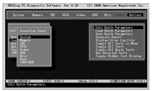
Choose the number of times that you want to run the AMIDiag tests on the associated AMIDiag menus. You can run each test up to 255 times. If you have set the Passbound parameters (see the previous screen) to 5 and you set the repeat count to 5, the test will be run a total of 25 times.
